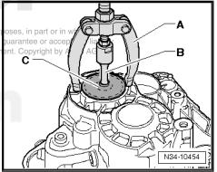
Remove the locking ring -C- from the input shaft grooved ball bearing as follows:
