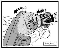
Remove the shift cable lock washer -1- from the gearshift lever
