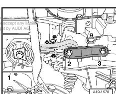
Remove the bolts -1 and 2- and the primary catalytic converter bracket.
