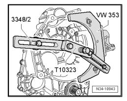
Install the input shaft -1- together and the selector rod for 5th and 6th gears into the clutch housing.
