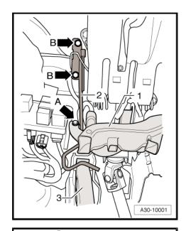
Remove the nut -2- and bolt -5- and then remove the clutch pedal -1- from the bracket -3-.
