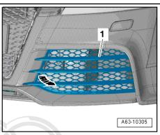
Remove the bolt -1- and the air guide.
