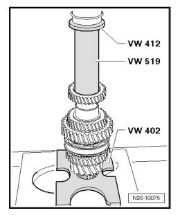
Installing the Inner Race/Tapered Roller Bearing in the Transmission Housing.
