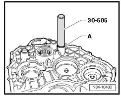
Remove the Input Shaft Seal.
