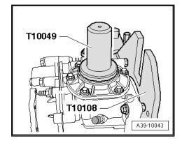
Fill the space between the sealing and dust lip half way with sealing grease -G 052 128 A1-.
