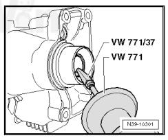
Pry out the stub shaft seal on the drive axle side.
