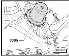
Fill the area between the sealing lip and dust lip -arrow- halfway with sealing grease -G 052 128 A1- .
