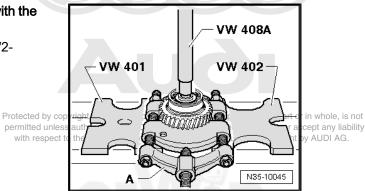
Remove the 5th and 6th Gear Synchronizer Hub/Locking Collar with the 5th Gear Wheel.
