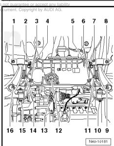
Remove the left coolant pipe. Refer to  $\Rightarrow$  Engine Mechanical; Rep. Gr. 19; Removal and Installation .
