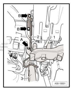
Remove the nut -2- and the bolt -5- and then remove the clutch pedal -1- from the bracket -3-.
