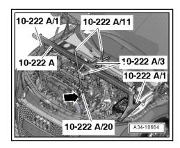
Remove the engine/transmission connecting bolts -1-.
