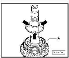
Installed Position: Synchronizer Ring -A- (3rd gear inner race)
