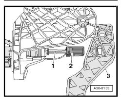
Install the over-center spring -2- in the bracket from the top.
