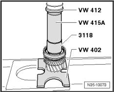
Installation Position, 3rd Gear Outer Race.
