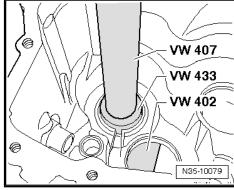
Removing the Inner Race/Tapered Roller Bearing in the Clutch Housing.
