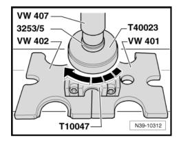
Secure the stub shaft with the countersunk bolt and tighten the bolt to the tightening specification, ⇒ Item 12 (page 179).
