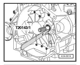
Install the Input Shaft Seal so that it is Flush.
