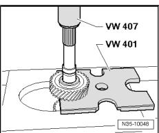
Installing 4th Gear Wheel.
