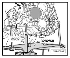
Install the -3282/34- into the hole in the transmission for the pendulum support bolt.
