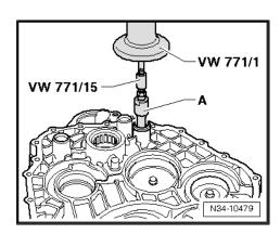
Install the Selector Rod Bushing -A- all the Way.
