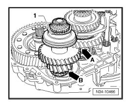
Installation Position; 3rd and 4th Gear Selector Rod ses, in part or in whole, in arantee or accept any lial
