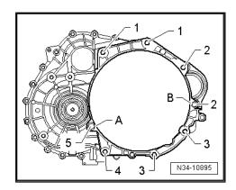
Remove the bolts -arrows- from the transmission mount.
