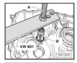
Installing the Outer Race/Tapered Roller Bearing into the Transmission Housing.
