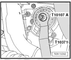
Remove the upper bolt -arrow- from the bevel box.
