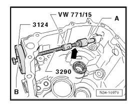
Installing the Gearshift Shaft Bearing Bushing -A- All the Way onto the Tool
