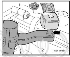
Remove the bolts -arrows-. Then remove the cable bracket from the transmission and tie it up to the left.
