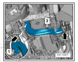
Remove the bolts -1, 2 and 3- and the bevel box bracket.
