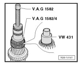
Installing the Inner Race/Tapered Roller Bearing in the Clutch Housing.
