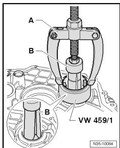
Installing Outer Race/Tapered Roller Bearing into the Clutch accept any I Housing with respect to the correctness of information in this document. Copyright by AUDI A
