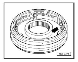
Pressing on Locking Collar/Synchronizer Hub for 3rd and 4th Gears.
