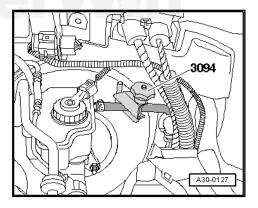
If there is a hose/line assembly between the clutch master cylinder and the clutch slave cylinder, then clamp the hose -A- with the -3094- .
