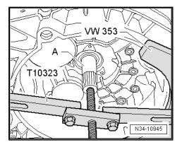
Bolt together the transmission housing and the clutch housing.
