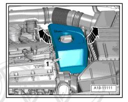
Remove the air filter housing. Refer to  $\Rightarrow$  Fuel Injection and Ignition; Rep. Gr. 24; Removal and Installation .
