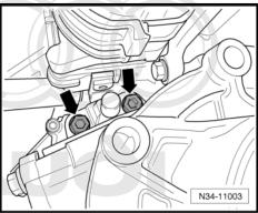
Protected by copyright. Copyi Remove the upper bolt -arrow- from the bevel poxted unless authorised by
