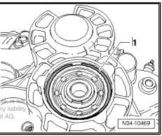
Remove the -T10323- for the input shaft -A-.
