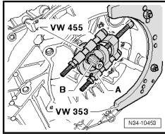
Remove the switching rockers for reverse gear -A-.
