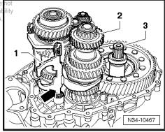
Lower the input shaft just enough -A- by turning the spindle on the -T10323- so that it remains slightly tensioned (lifted approx. 1 mm).
