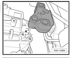
Align the -3282- with the -3282/60- in order to remove the "0A6" transmission.
