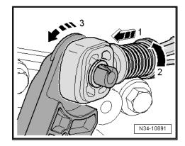
Remove the shift cable lock washer -1- from the gearshift lever -2- and then pull the shift cable off the lug -arrow-.
