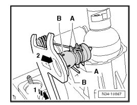
Place the shift housing with the shift lever guide into the larger cavity -arrow- in the -T10083- .
