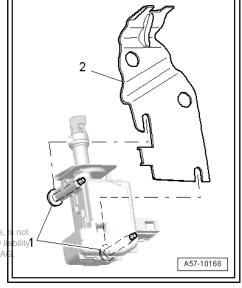
Guide emergency release -2- through clip -3- on motor -1-.
