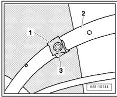
Remove retainer bolts on tensioning strap from rail »3«.
