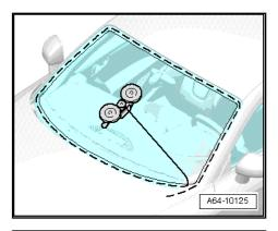
Move spooling tool as shown, and continue to cut out adhesive sealing material.
