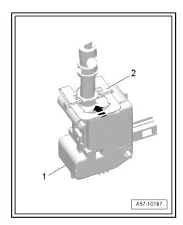
Insert motor in bracket -2- and tighten with bolts -1-.
