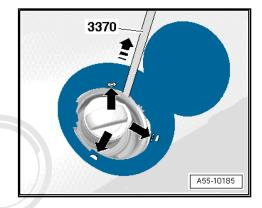
Unlock the locking mechanism -arrow- with the hook -T40207- or a hook made as an assisting tool of welding wire, for example.
