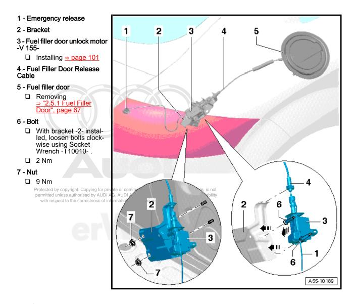
Fuel filler door emergency release cable routing
