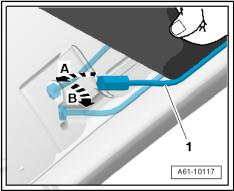
Engage spring -3- in eyes -arrow- on main guide -1- and rear tension cable -2-.
