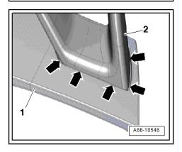
Tighten the screws -arrows- on the left and right with the specified torque. Refer to ⇒ Item 22 (page 225)
