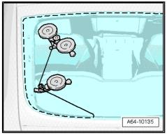
Remove idler pulley and continue cutting window free.
