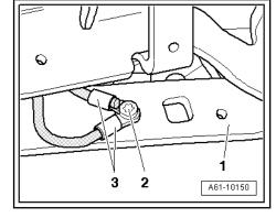
On angle bracket -1-, drill out rivet heads -arrows- for securing the cover and drive out rivet shafts.
