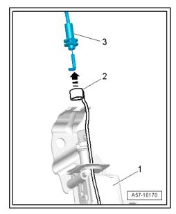
Insert cable -1- in operating rod -2- and turn until it engages audibly.
