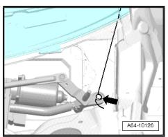
Secure beginning of cutting cord in spooling tool and cut out first area of adhesive (up to about center of windshield).
