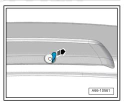
Clean all surfaces -arrows- that will later be in contact with double-sided adhesive tape with cleaning solution -D 009 401 04- .
