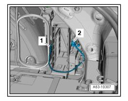
Unclip cover strip -2- on upper bumper -1- from the locking mechanisms -arrows - and remove.
