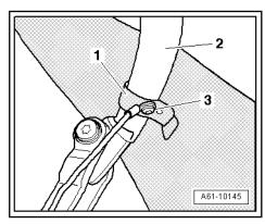
Remove bolt -3- on guide strap -1- as shown on roof guide
