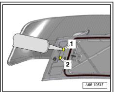
Use the glue cartridge from the installation kit to place an adhesive bead around the screw heads -arrows- of the left and right screws and spread.
