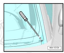
Lay cutting cord underneath and all around inside of windshield.
