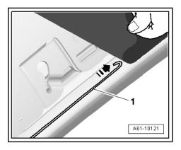
Engage the tension cable in the hook as shown and pull for-
