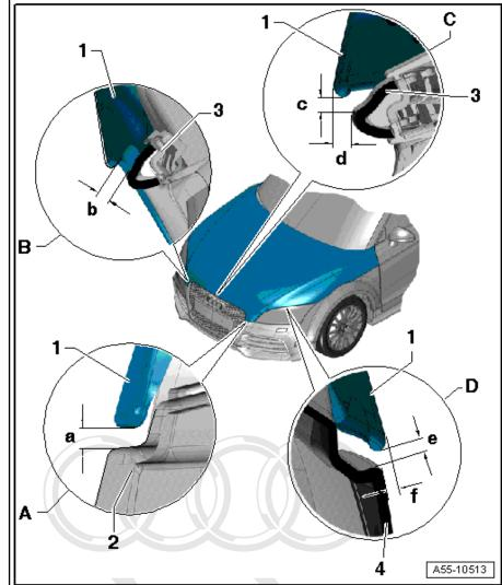
Protected by copyright. Copying for private or commercial purposes, in part or in whole, is not **Gap Dimensions of Hood to Fender Front Door** horised by AUDI AG. AUDI AG does not guarantee or accept any liability with respect to the correctness of information in this document. Copyright by AUDI AG.
