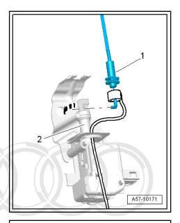
Slide emergency release cap -3- onto operating rod and press cable bracket -2- into bracket mount -arrow-.
