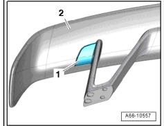
Clean the base plate and spoiler-center part of the adhesion area-arrow- with cleaning solution -D 009 401 04- .
