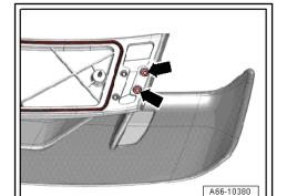
Check the gap size -arrows- between spoiler base plate -1and spoiler center part -2-, center if necessary.
