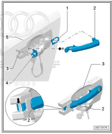
When installing door handle -1-, rear end must slide into mounting bracket in -direction of arrow- as shown.
