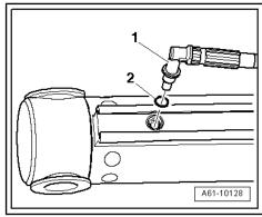
Carefully remove sealing ring -1- using a small hook -2- if necessary without damaging -3- cylinder.
