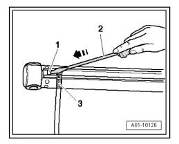
Remove connecting piece -1- from cylinder using sealing ring -2-.
