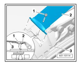
Remove retainer bolts on tensioning strap from rail »1« as shown.
