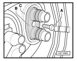
Remove left footwell vent -A- (driver side). Refer to⇒ Body Interior; Rep. Gr. 68; Removal and Installation.
