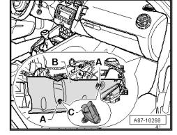
Slide the cover -B- in direction of arrow -C- and remove it.
