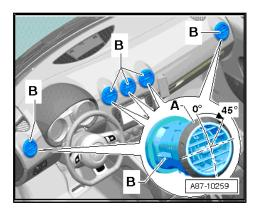
Attach, for example, -3438- -A- on rear end -C- of instrument panel vent -B-.
