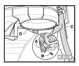
Disengage both flanges for coolant pipes to heater core -Aand for expansion valve (to evaporator) -B- from passthroughs of grommet -C-.
