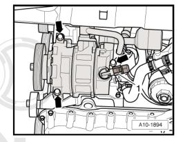
Before securing A/C compressor, check seating of both alignment bushings -arrows- in bracket or A/C compressor.
