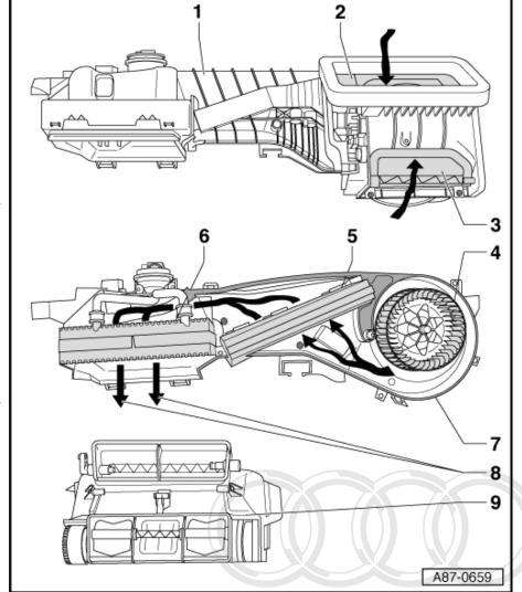
There are different versions of the dust and pollen filter (with and without an activated charcoal insert). Refer to the Electronic Parts Catalog (ETKA). An Audi TT with A/C has a dust and pollen filter with an activated charcoal insert is installed. An Audi TT without A/C has a dust and pollen filter without the activated charcoal insert.
