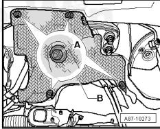
Mark arrangement of coolant hoses -A- and -B-.
