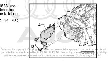
Mark connector -C- to Left Temperature Door Motor -V158-(danger of interchange with other connectors of same construction).
