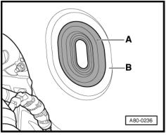
Have the second mechanic (working from engine compartment) guide both flanges for coolant pipes to heater core -Aand for expansion valve (to evaporator) -B- through passthroughs of grommet -C- when inserting heating & A/C unit.
