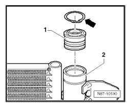
Remove the dryer bag using a commercially available pick-up tool -in direction of arrow- from the condenser.
