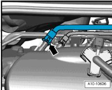
Remove components that block access to the coolant hoses
