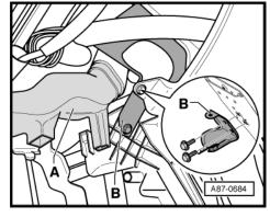
Remove the bracket -B-. Refer to ⇒ Body Interior; Rep. Gr. 68; Removal and Installation.
