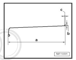
Hook the welding wire to the strainer exactly as illustrated to prevent damaging the condenser.
