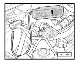
Leak Detection System VAS 6201
