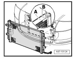
If condenser is replaced, observe flat pipe dimensions. If a condenser with different dimensions is installed, the sticker -A- specifying the capacity for refrigerant R134a is also to be replaced, or the old capacity specification is to be removed and the new capacity is to be noted, for example, using a waterproof marker. Refer to Electronic Parts Catalog.
