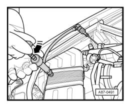
Leak Detection Additive With Filled Refrigerant Circuit, Filling
