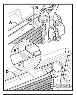
If condenser is replaced, observe flat pipe dimensions. If a condenser with different dimensions is installed, the sticker -A- specifying the capacity for refrigerant R134a is also to be replaced, or the old capacity specification is to be removed and the new capacity is to be noted, for example, using a waterproof marker. Refer to Electronic Parts Catalog (ETKA).
