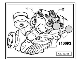
Tighten the bolts -arrows- to the tightening specification, refer to  $\Rightarrow$  Item 1 (page 39).
