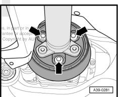
Remove the bolts -arrows- for the center bearing and the heat shield. Then remove the heat shield.
