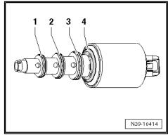
Place the new cover -2- on the control module -1-.
