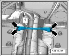
Counterhold the rear final drive with the -T10172- and -T10172/5- when loosening or tightening the driveshaft.
