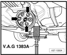
Install driveshaft on final drive so that both markings -arrows- align.
