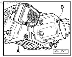
Remove the fastening bolts -arrows- and remove the Haldex clutch from the rear final drive.
