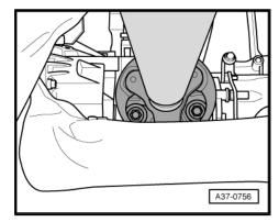
Remove the bolts -1 to 3- and remove the pendulum support.
