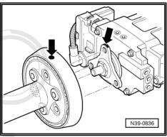
Counterhold using the -T10172- and remove the driveshaft bolts -arrows- from the rear final drive.
