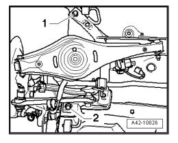
Remove the crossmember -1- -arrows-. Refer to "All Wheel Drive (AWD)" in ⇒ Suspension, Wheels, Steering; Rep. Gr.
