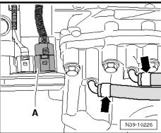
Remove both of the transmission bleeder hoses -arrows- from the subframe.
