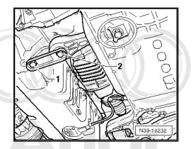
Press the engine and transmission forward and secure the position with a suitable piece of wood -A-.
