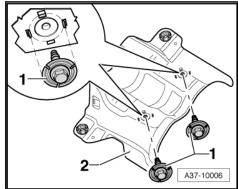
Tighten the pendulum support with new bolts. For the correct tightening specifications. Refer to ⇒ Suspension, Wheels, Steering; Rep. Gr. 40; Specifications.
