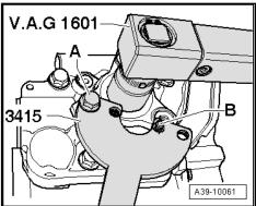
Remove the oil filter unit.
