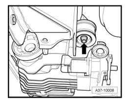
Remove the pump connector -arrow- from the control module.
