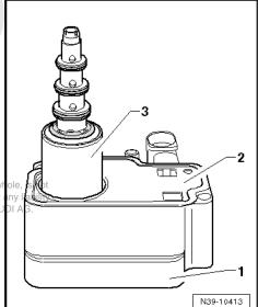
Insert the Haldex clutch control valve -3- into the control module -1-.
