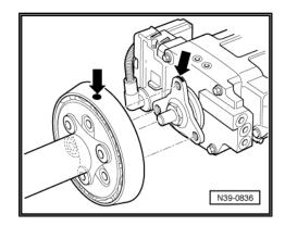
Attach the driveshaft with flexible disc to the rear final drive -arrows-. Tightening specification ⇒ Item 22 (page 110)
