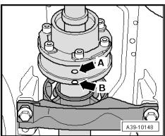
Attach the front driveshaft tube to the rear driveshaft tube -arrows-. Tightening specification ⇒ Item 7 (page 109).
