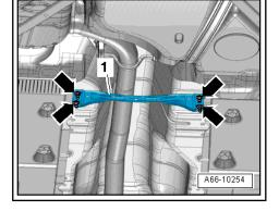
Remove bolts -1 and 3- and remove diagonal braces -2-.
