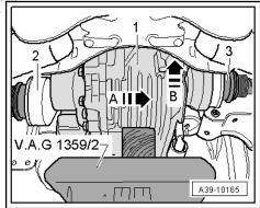
Use the strap -B- to keep the rear final drive -1- from falling.
