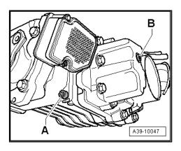
Lower the final drive slightly. The fastening bolt -arrow- on the front final drive mounting bracket must be unscrewed approximately 7 turns for this purpose.
