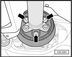
When removing and installing the driveshaft, be careful not to damage the bushing -arrow-.
