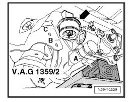
Disconnect the connector -A- on the All Wheel Drive (AWD) control module -J492- .
