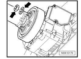
Counterhold the rear final drive with the -T10172- and -T10172/5- when loosening or tightening the driveshaft.
