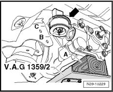
Disconnect the harness connector -A- on the All Wheel Drive (AWD) control module -J492- .
