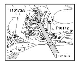
Remove the bolts -2 and 3- for the pendulum support.
