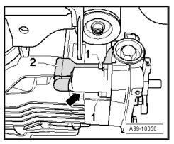
Remove the fastening bolt -arrow- at the front mounting bracket
