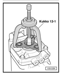
Remove the seal using an -VW 681- .
