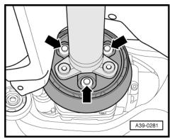
Carefully remove the rear driveshaft tube from the flange/driveshaft centering pins on final drive.
