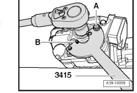
Remove the driveshaft flange. Use a three arm puller (for example, Kukko 12-1) if difficult to access.
