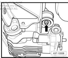
Clip the wiring harness to the Haldex clutch securely and place the connector -arrow- on the control module.
