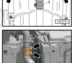
Remove the pendulum support bolts -1 and 2-.
