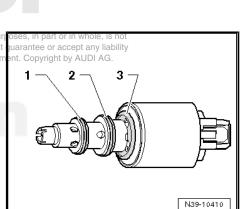
Replace the O-ring -arrow A- on pressure sensor.
