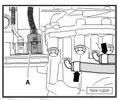
Remove both of the transmission bleeder hoses -arrows- from the subframe.
