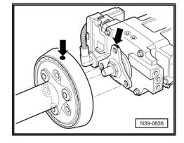
Remove the rear driveshaft tube with the flexible disc and vibration damper from the rear final drive -arrows-.
