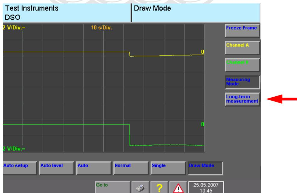
image 5-18 “DSO” mask with operating button for setting long-term measurement
