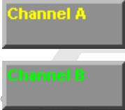
Press the operating button “Channel A” or “Channel B” to display the operating functions for “Channel”, “Measurement range”, “Coupling”, “Min/Max” and “Measurement preset” below the display field and thus be able to access them for this channel.
