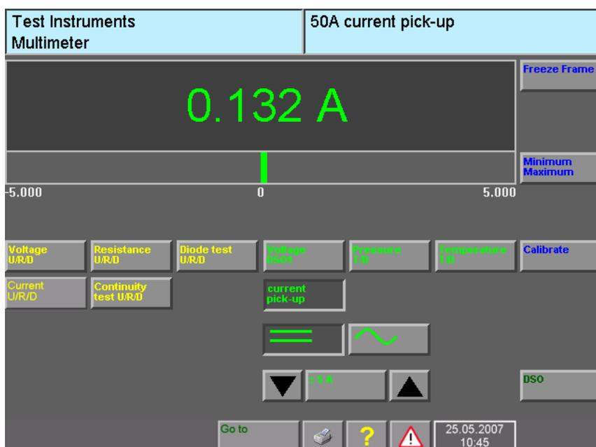
image 5-5 "Multimeter" mask: current measurement with the 50 A current pick-up
